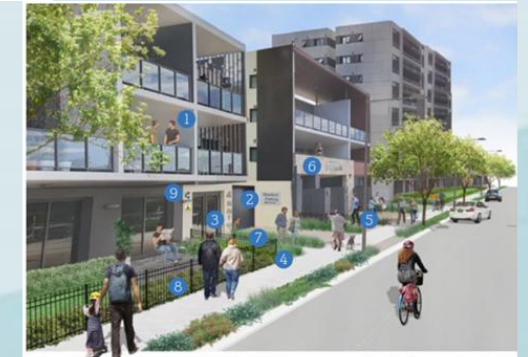
Figure 1- Mixed-use streetscape: 1) Signage to encourage orientation and mixed use of spaces; 2) Visibility from private buildings and activities on public spaces, to encourage informal surveillance; 3) Visible and accessible waste bins, for urban image care and management; 4) Activation of public space and areas near commercial activities to encourage informal surveillance; 5) Clear use of spaces, streetscape integrated with commercial activities to enhance sense of territoriality; 6) Lighting and CCTV for formal surveillance of spaces.
