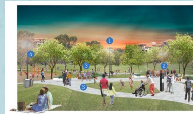
Figure 2. Landscape of a public open space: 1) Lighting to encourage activities even in the evening hours and increase the sense of safety; 2) Signage, to encourage orientation; 3) Clear sight lines across the park and in the different spaces of the park (paths, play areas, etc.) to encourage informal surveillance; 4) CCTV for formal surveillance; 5) Paving used to indicate pedestrian routes, to increase the legibility of the spaces.
